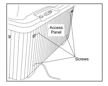
If the spa will be stored for any period of time, place the power cord inside the spa before re-attaching the access cover.
